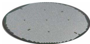
400,000 I/O's, 80µm SnAgCu
